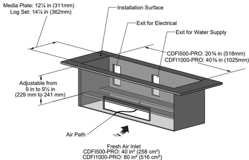
2. If connecting to plumbing, complete the water connection according to the instructions in the 'Cassette Plumbing' section (page 10).
