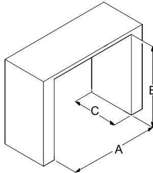
2. Make sure there is clearance for air circulation beneath the unit.
