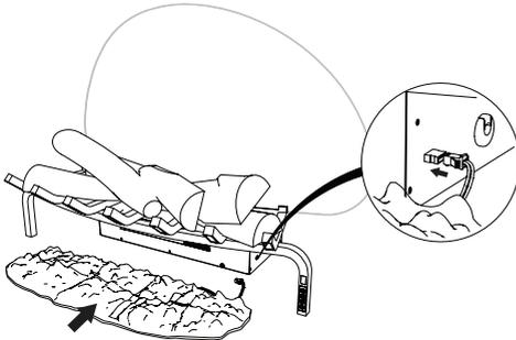
4. Install the Mirage™ Flame Panel by inserting the bottom edge into the tabs between the back log and grate log assemblies.
